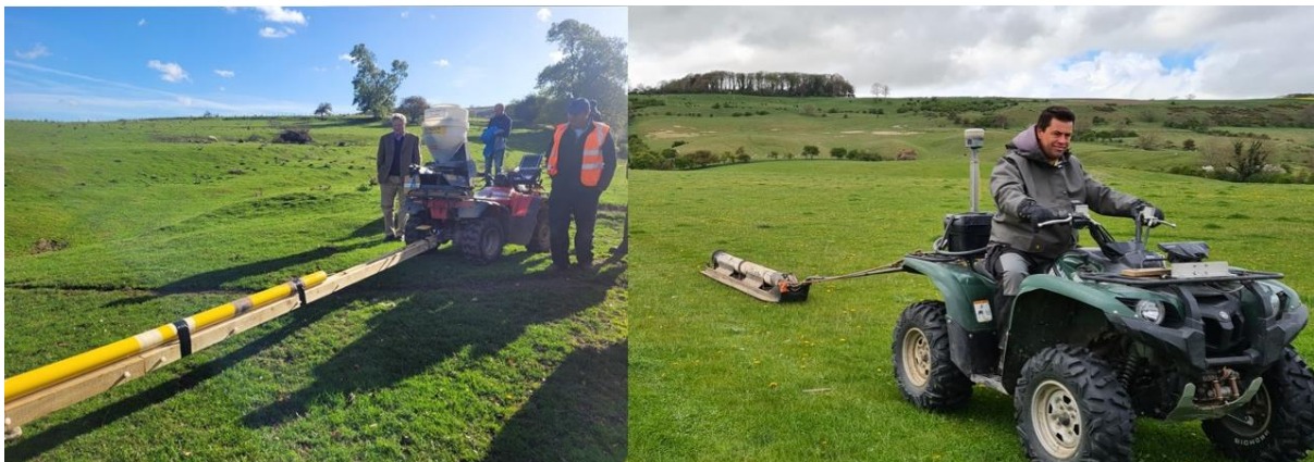
Figure 4 FDEM data collection in the field – similarities and differences: agricultural sensor set-up on the left (Photo: Rachel Opitz), archaeological prospection on the right (Photo Philippe De Smedt).
