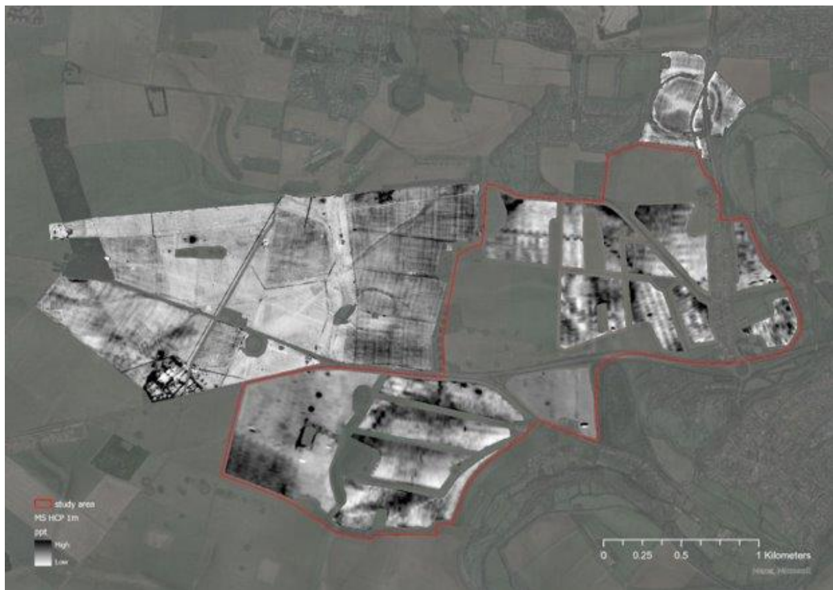
Figure 4 Case study area (red outline) with agricultural FDEM magnetic data collected by Soyl Ltd, side-by-side with archaeological prospection data – University of Ghent FDEM conductivity data (De Smedt et al. 2022 and Gaffney et al. 2018).
