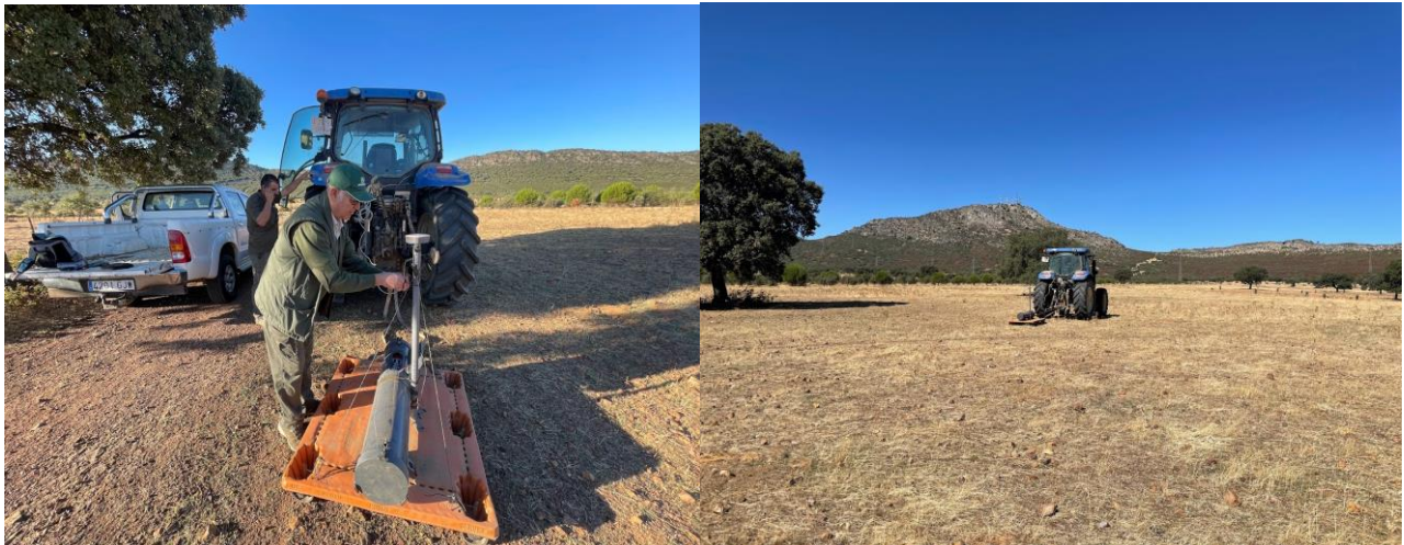
EMI mapping with a EM38Mk2 using a tractor towed system
